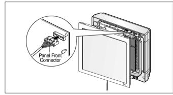
3. Screw up panel front, and suspend the hook of panel front in the groove.
